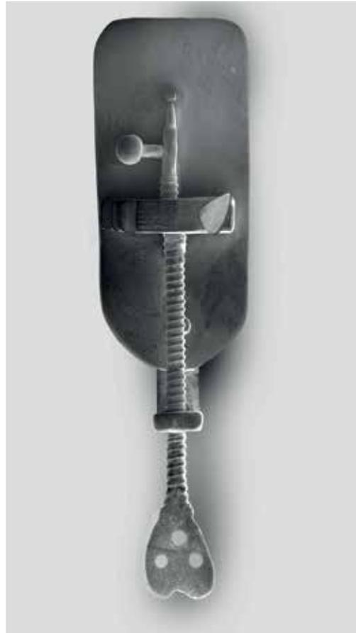
**Figure 5:** This SEM macrograph was assembled from 70 frames taken with the Hitachi S-3400N variable-pressure microscope at the Cavendish Laboratory, Cambridge. It correlates with the digital camera image from the Olympus E-500 camera with Zuiko Digital 35mm macro lens and assembled from 40 frames (fig 4). These images measure 27,000 pixels (2.18 cm) long.
