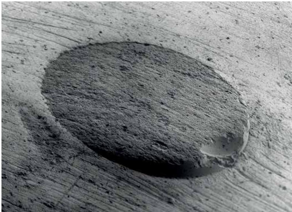
**Figure 11:** Severe abrasion characterises the side of the lens facing towards the observer. This surface has been ground flat and conchoidal fracture is also evident. Leeuwenhoek was known to insist on the highest standards for his lenses and the only reasonable explanation for this remarkable result is that it was deliberately destroyed by its maker.
