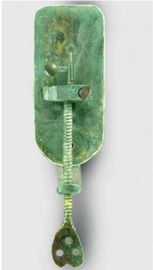
**Figure 4:** The twelfth microscope was excavated from mud that had been dredged from the canals of Delft and was advertised on eBay. The vendor believed it to be a "weird kind of drawing instrument" and for a time he told the purchaser that it had been lost. The brass plates measure 17 x 40 mm though the lens has been severely abraded. This was the first to be examined by SEM.
