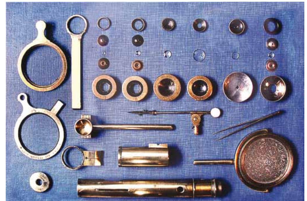
Fig. 7. Component parts of the Linnean Society microscope are here displayed in disassembled state. The stage assembly (left) and body components (below) can be identified. The six lenses (top) are held in place within the brass lens holders by retaining cups; and the aperture of the smaller lenses, being of higher power, were all restricted by means of perforated steel stops. Although this reduces resolution, it significantly increases image contrast.
