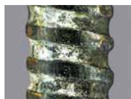
FIGURE 10 The use of a loupe or hand lens can provide useful evidence of the thread structure. This is a selective enlargement from our studies of the Camacho/Pallas microscope with a Zuiko Digital 35mm macro lens and Olympus E-500 camera which resolves sufficient detail to conclude that the thread was not produced by a post-industrial die.
