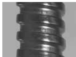
FIGURE 5 The rolling of a thread by Leeuwenhoek would ideally produce a square contour as modelled by this modern example of a steel tube. Producing a thread by rolling involves apparatus that requires less precision than manufacturing a high-tensile tap and die of the industrial era. The threaded portion of a rod increases in diameter during the rolling process.
