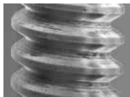
FIGURE 3 The long screw of the replica by Chris Kirby has squared crest and root, closer to that of a Leeuwenhoek microscope. This has been cut with a UNC die (fig 13) and Kirby selected a brass rod that has a diameter 0.33 mm smaller than that for which the die was manufactured. This exaggerates the flattened crest. Same scale as Fig 2
