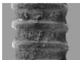
FIGURE 8 Present-day rolled threads are used for securing the spokes of bicycle wheels, and this well-used example provides a fitting comparison with the mud-encrusted thread in Fig 7. The characteristic squared profile is evident, with broad crest and root (Fig 12). Note also the deformation of the crest that is seen more clearly in the Leeuwenhoek microscope.
