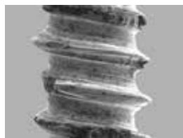
FIGURE 4 In Utrecht, the best of the microscopes attributed to Leeuwenhoek magnifies 266x and replicas of this remarkable instrument were made for some years by Mr. Hansen van Walle of Antwerp, who kindly donated one to the author. Under the SEM the cutting of the thread can be observed, and fragments of brass have been broken away by the industrial die.
