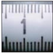
The field of view with the 10x lens covers 20 mm.
