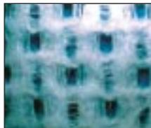
**The structure of non-woven fabric under the 10x lens.**
