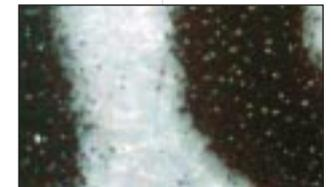
**At 200x the grains of toner are unmistakable. A copy.**
