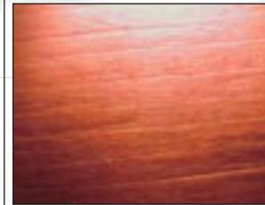
Here is the view of a pine door under the 10x objective.
