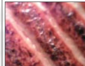
At 60x the truth is revealed - the 'oak' is made of plastic.
