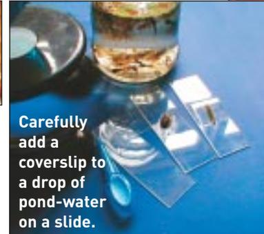
**Carefully add a coverslip to a drop of pond-water on a slide.**
