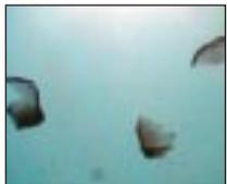
**Fragments of cork cut with a cutting-knife 10x magnified.**
