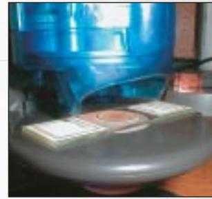
**Using the stage without clips aids positioning a slide.**
