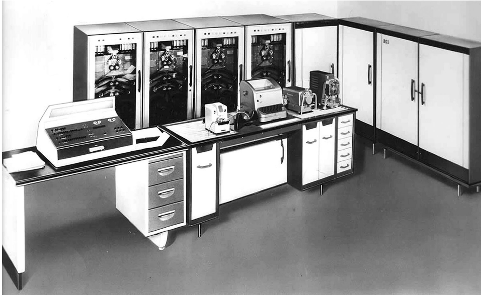
The first computer I programmed was this Elliott 803 at the Cardiff Institute of Science and Technology in 1962. It occupied an entire room to itself, and a 1,000 ft (305 m) spool of punched tape stored just 1.3 MB of data. Only one of the original computers is still fully operational, at the museum of Bletchley Park, U.K., where the World War II codebreaking computers have also been restored.
