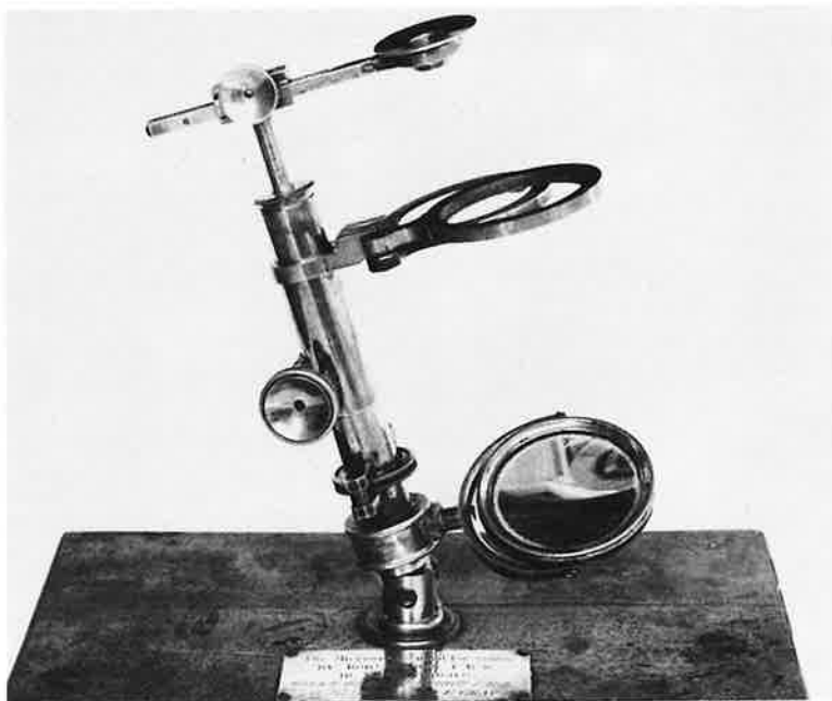
Figure 2. Robert Brown's microscope at Kew represents a type similar to that produced by Bancks (see Figure 3). But there is an added feature: the substage mirror housing is mounted on a rotating collar which enable lateral lighting to be more easily utilised. Brown dispensed with a substage condenser, preferring a double-sided mirror instead. The lens unit is shown in its fitted position here.
